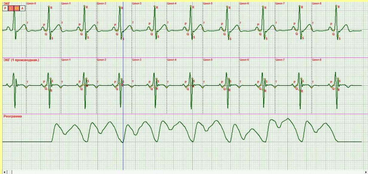
**Figure 1.** ECG, ECG first-order derivative and Rheogram recorded with the PC-assisted device Cardiocode.
